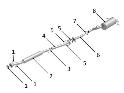
(Carefully read all instructions before installation) Disconnect the vehicle's battery before removal of the OEM exhaust system. This will prevent electrical accidents and will reset the computer if it applies to the vehicle. Remove existing exhaust system from the vehicle. Only remove parts that will be replaced. Clean existing flange with a wire brush to ensure proper sealing.
